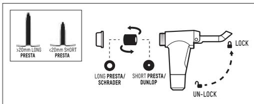
Press pump head onto valve. Flip lever into the lock position.
