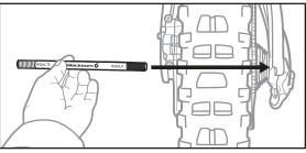
Insert axle through non drive side side of frame. The axle threads into the drive side of the bike. Be sure the correct thread pitch side is inserted into threaded side of bike frame.
