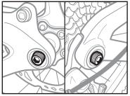
Use 5 mm hex key to screw in the axle so equal portions of the axle are exposed on either side of the bike frame.
