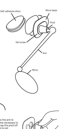
FOR ADJUSTMENT: A set screw inside the pivot enables the arm to keep the mirror in your selected position. It may become necessary to tighten this screw with a 3mm allen wrench. Simply snap the pivot off the mirror base and tighten from the inside. Be careful to not overtighten as it may strip the threads inside the pivot.
